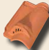
171F01 Aerator tile It is useful to keep the roof ventilated. You need one aerator tile every 25 m 2 of roof.
